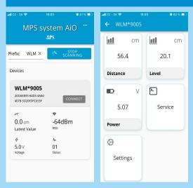
Scan for nearby compatible sensors. Display current measurements. Display short-term measurement history in grafical and tabular form. Change sensor setttings. Upload firmware.
