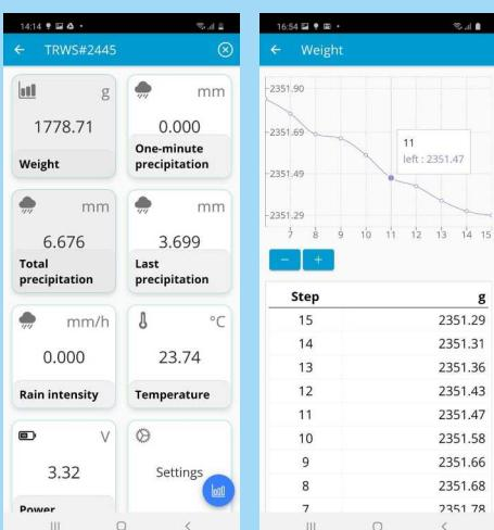
Scan for nearby compatible sensors. Display current measurements. Display short-term measurement history in grafical and tabular form. Change sensor settings. Upload firmware.
