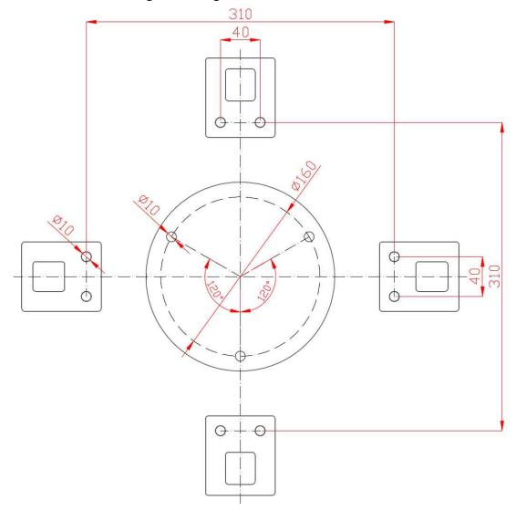
• Secure **11 pcs** of **M8 threaded rods** using a chemical anchor. Make sure that the threaded rod protrudes at least 15 mm above the concrete level.
